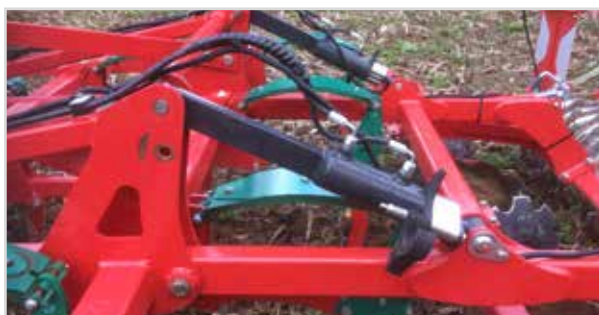
The rear roller of the Enduro is not linked via parallelogram and is adjusted hydraulically via spacers.
